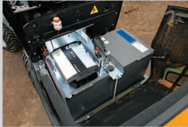
The G2700E models are easy to maintain because service points are easy to access. Hydraulic system and battery are freely accessible via the easy-to-use open service valves. This ensures that daily checks and maintenance can be carried out quickly and safely.
